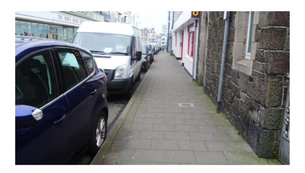
42 An uncontrolled crossing across Main Street is provided outside the White House. The tactile paving does not contrast sufficiently with the surrounding paving.
