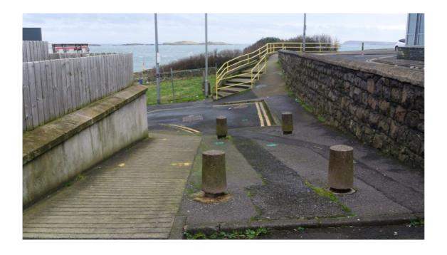
Current crossing facilities at the corner of Bath Street/Terrace are in need of upgrading including correctly installed tactile paving.
