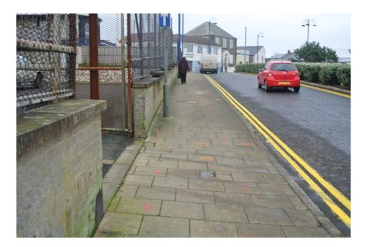
The footway broadens around the health centre on Dunluce Avenue. An uncontrolled crossing is provided here with access to the car park. The tactile paving does not contrast sufficiently with the surrounding paving. The positioning of a bin partially blocks the crossing on the car park side.
