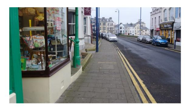
An uncontrolled crossing is provided across the junction with Bath Street. There are significant crossfalls on the footway around this junction. Bins and A Boards obstruct narrow pavements on Main Street after the crossing.
