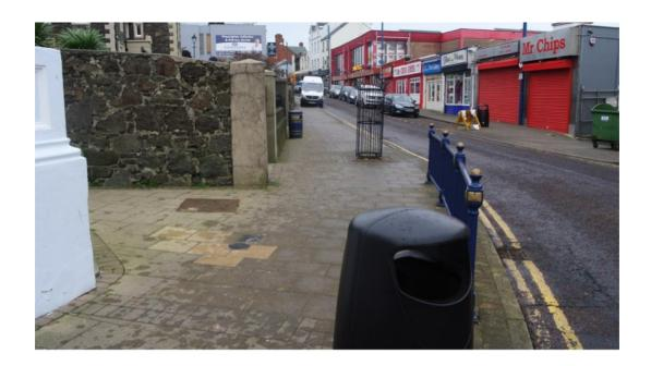
There is an uncontrolled crossing at the church to the eastern side of Main Street. Tactile paving is provided but does not contrast sufficiently with surrounding paving.
