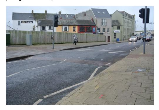
The broad footway continues along the western side of Dunluce Avenue until a side street is reached. An uncontrolled crossing has been provided with tactile paving. However multiple bollards (designed to prevent pavement parking) create significant hazards for people with a visual impairment in particular. The pavement narrows considerably after this point.
