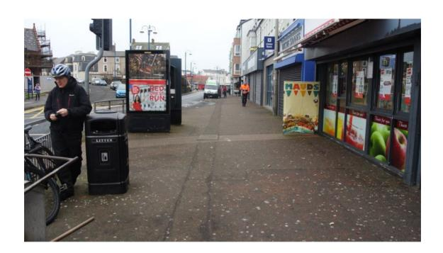
An uncontrolled crossing has been provided to enable people to access the western footway and Mark Street further along Eglington Street. This is a good example of an uncontrolled crossing although parking does obstruct sight lines for pedestrians and drivers.
