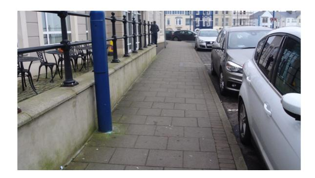
There is an uncontrolled crossing across Main Street just before the junctions with Causeway View and Mark Street. The tactile paving does not contrast sufficiently with the surrounding paving.
