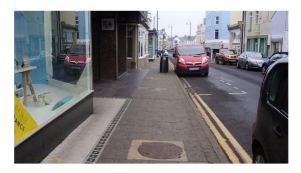
An uncontrolled crossing across Main Street is provided approaching the junction with Bath Street. The tactile paving does not contrast sufficiently with the surrounding paving.
