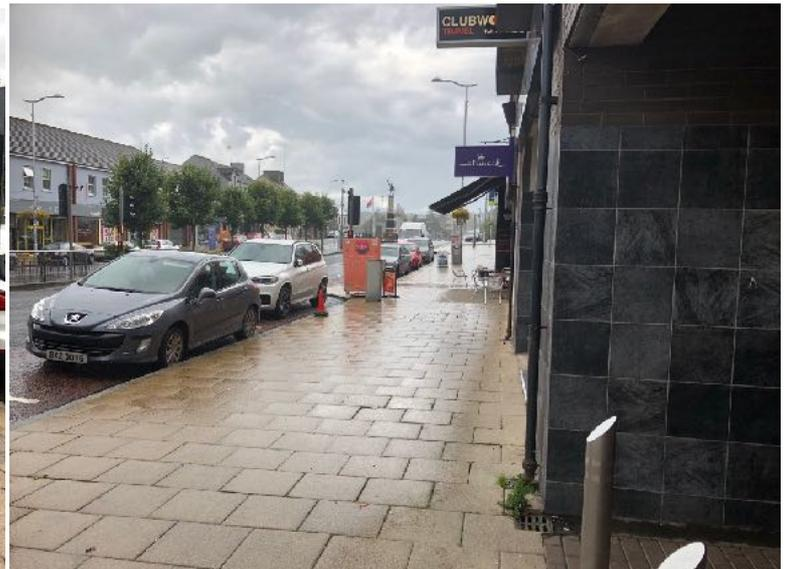
The Mall provides a linkage between the car park on Commercial Road and Newry Street. Currently the area is uninviting (despite floral displays). Surfaces are uneven in places and bollards at the Newry Street end do not include a visibility strip.
