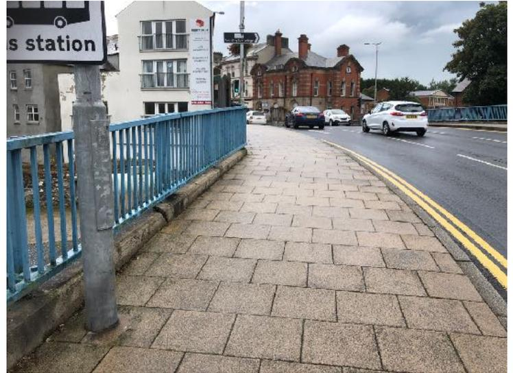
There is a controlled crossing across Huntly Road at its junction with Bridge Street and Church Square. The positioning of a lighting column on the northern side of the crossing obstructs access towards Church Square. Pedestrian railings emphasise the impact of traffic in the area.
