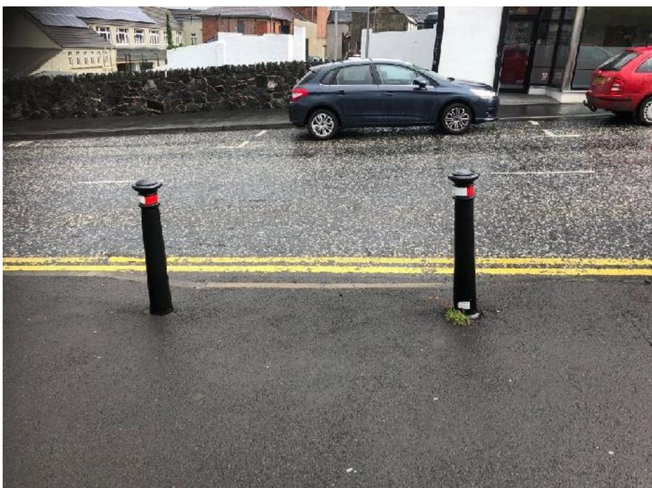
There is an uncontrolled crossing across the junction with Victoria Street. No tactile paving has been provided and the entrance to cinema on the northern side of the crossing obstructs access.
