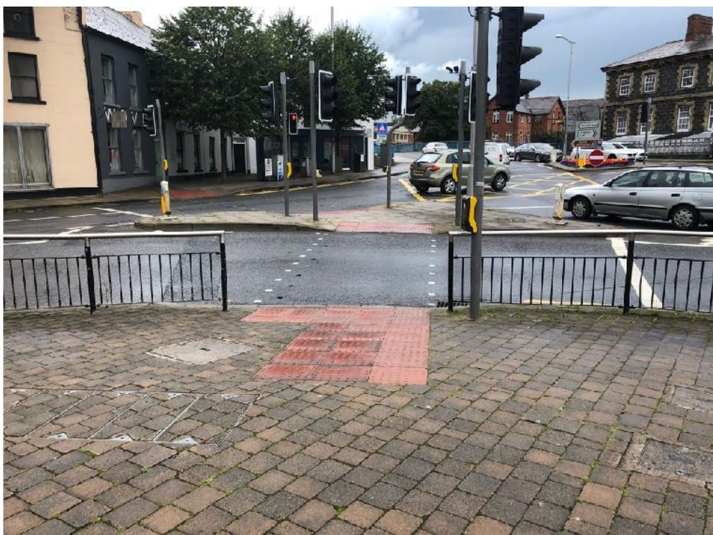
Footways on Windsor Terrace are narrower and in poorer condition compared to Church Square. A junction without tactile paving and A Boards create potential hazards on the southern footway.
