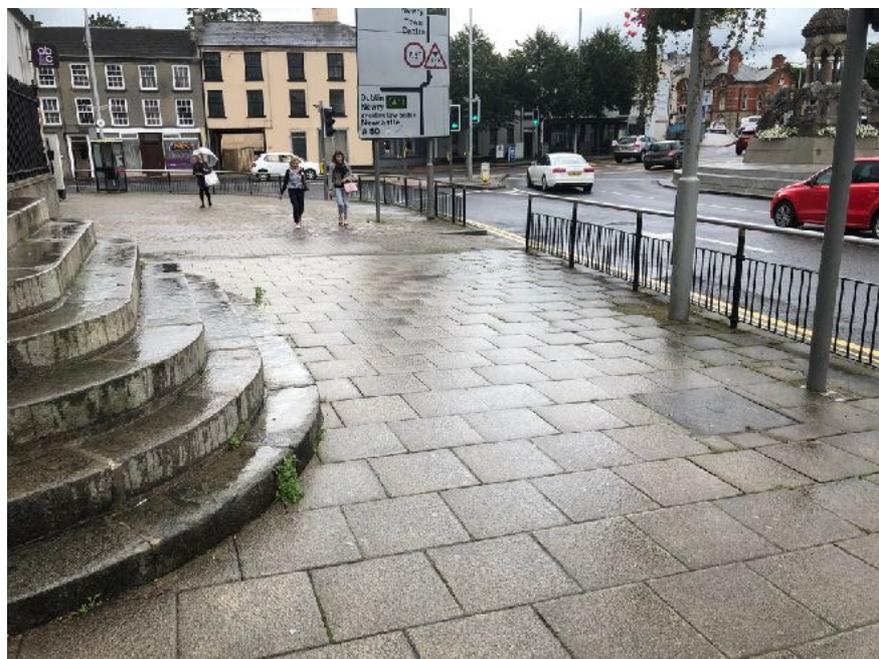
There is a controlled crossing at the junction of Church Street and Windsor Terrace. The crossing is split with a traffic island at its mid point. Tactile paving and controlled crossings have been positioned correctly, although the tactile tail at the northern side does not extend to the building line.
