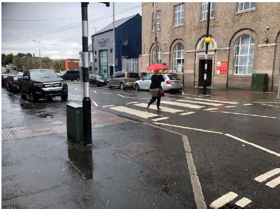
The southern footway on Scarva Street is narrow and uneven in places. Bins and shop displays on the pavement create potential hazards.
