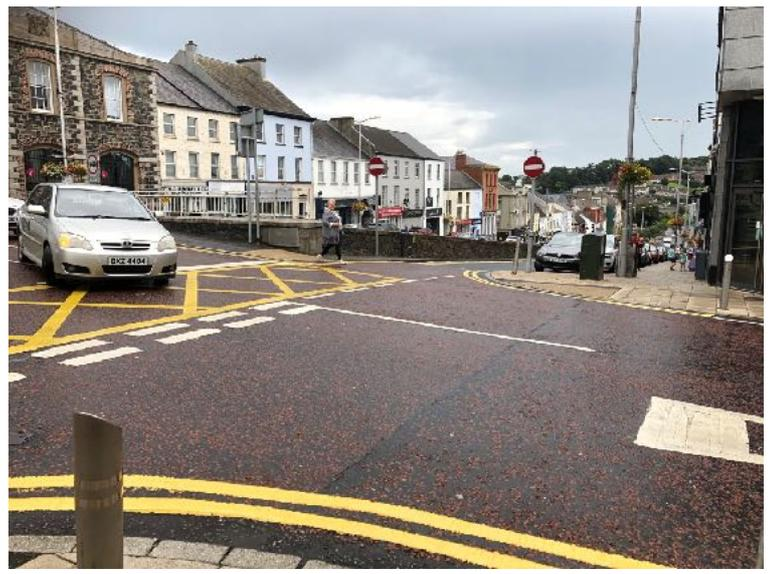
A series of uncontrolled crossings have been provided for pedestrians to cross the streets adjacent to the bridge. Stick down tactile tiles have been used on the bridge because of its listed status.
