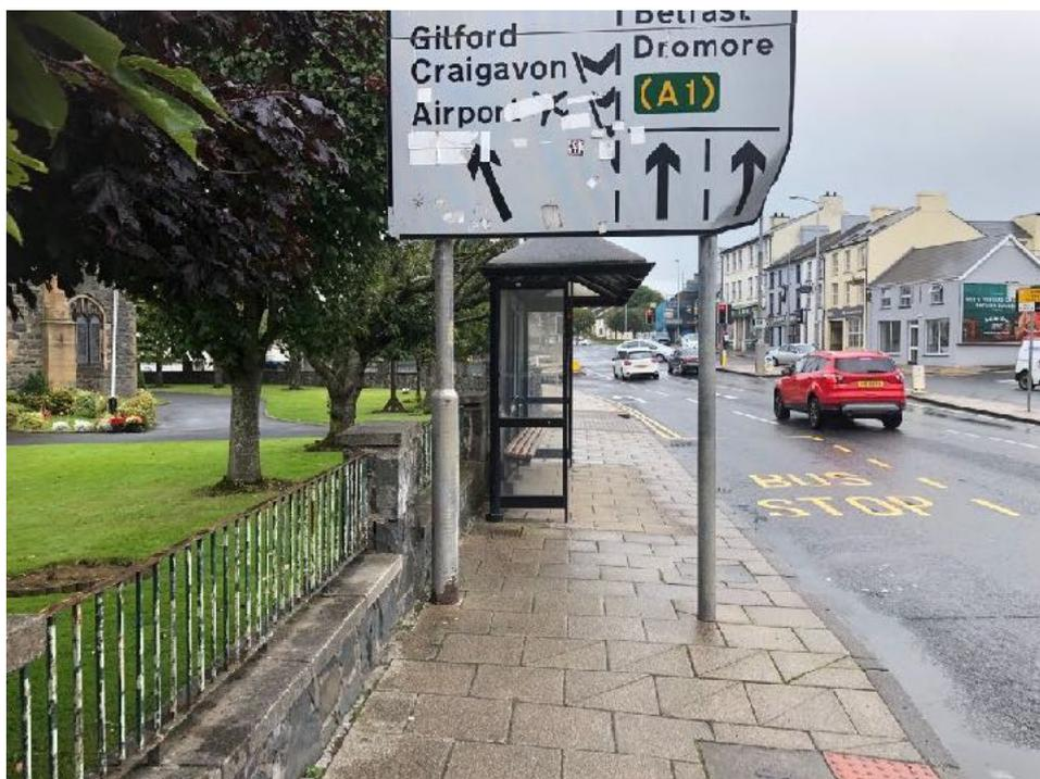
The vehicle entrance to Seapatrck Parish Church near the junction with Church Street has been constructed with a raised table with variable kerb shows at either side of the footway and no tactile paving, presenting significant hazards for disabled people.
