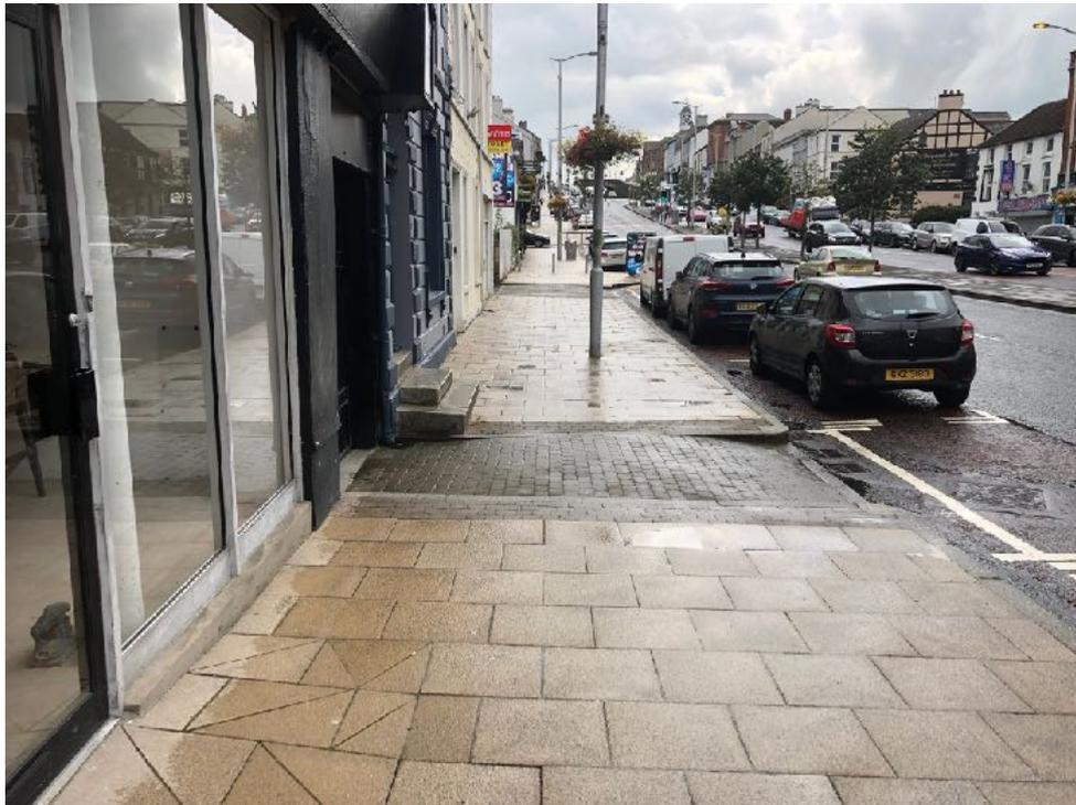
There is an uncontrolled crossing across the junction with Bridge Street East. The tactile paving does not contrast sufficiently with the surrounding pavement and lacks sufficient depth of tile on the southern side of the junction.
