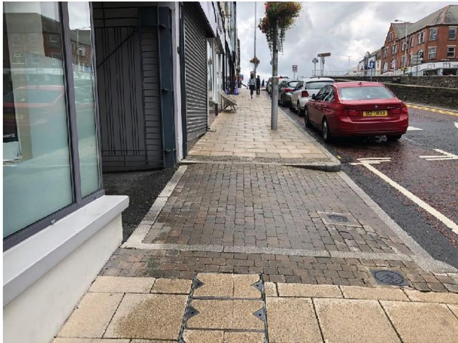
The western footway on Bridge Street is partially obstructed by ramped access to a B1 listed building close to the junction with Huntly Road and Church Square. Further street clutter impacts on access in the area.
