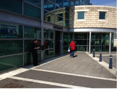
The station forecourt is cobbled and has constant vehicle movements. Signs encourage pedestrians not to use this area. Bollards mark out the boundary between the forecourt and pedestrian routes. The bollards would benefit from a stronger contrasting band.
