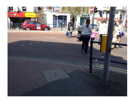
There is a traffic island at this crossing. The use of tactile paving here is unconventional and could be confusing for people with a visual impairment. Again some tactile paving is damaged and loose.
