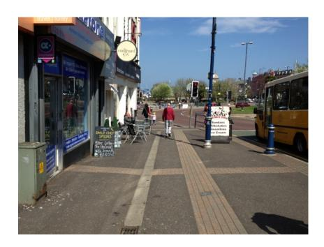
There is a controlled crossing at the northern end of Main Street. There is non-standard use of tactile paving as well as damage to the paving slabs presenting a potential trip hazard.
