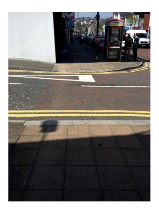
There is a controlled crossing at the junction with Bingham Street. There is a non-standard use of tactile paving. There are problems with the use of tactile paving on the associated traffic island (see 43).
