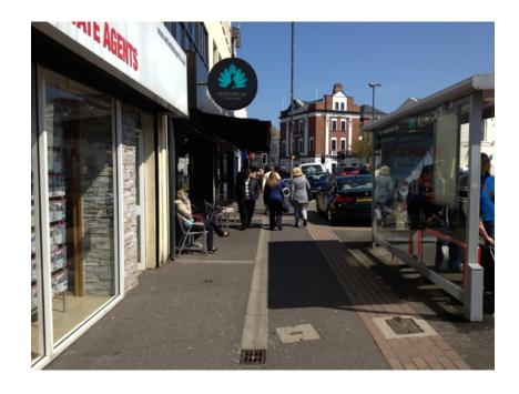
There is an in-line uncontrolled crossing at the junction of Market Street. A dropped kerb is provided but there is no tactile paving.
