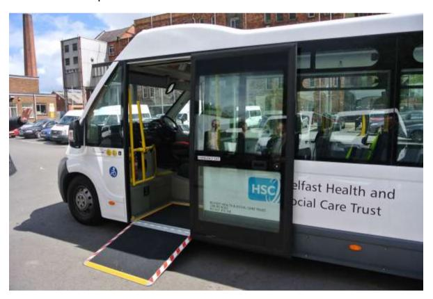
There is level access throughout the interior of the vehicle with tracking which allows flexibility in seat configuration. This means for example that a wheelchair user can sit with other passengers at the front of the vehicle rather than be restricted to the back of the vehicle as is often the case with high-floor vehicles.
