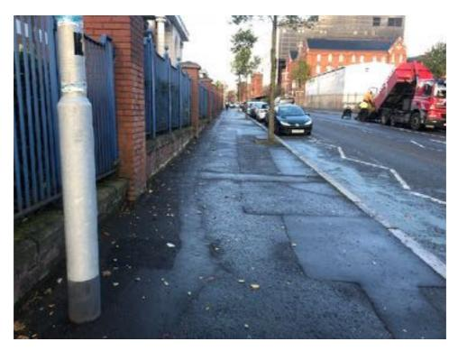
There is an in-line uncontrolled crossing across the junction with Hopewell Street. An additional line of tiles is required to meet tactile paving standards. The carriageway surface is rough and uneven.
