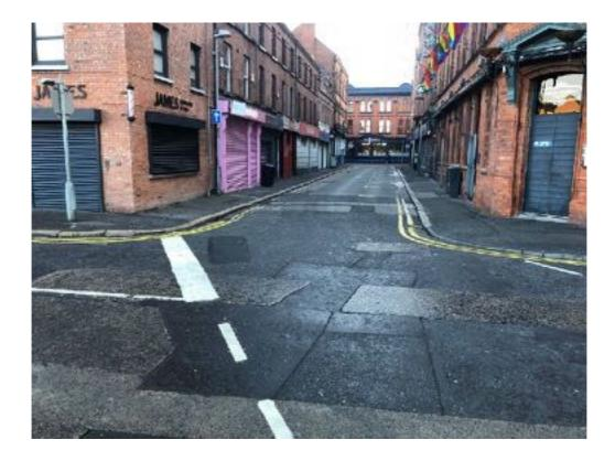
The northern footway on Union Street is narrow and in poor condition with large bins further reducing footway width.
