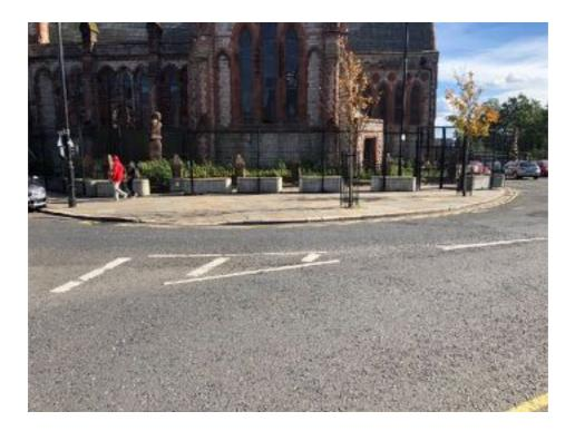
There is an in-line uncontrolled crossing across the junction with Denmark Street. The contrast between paving and the tactile on the southern section is poor. The crossing distance may present an issue for some given traffic levels in the area. There is a case for the provision of a pedestrian refuge at the mid point of the crossing.
