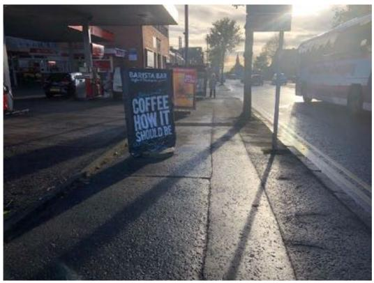
The kerbs are dropped at the garage exit but there is no tactile paving provided to warn pedestrians with a visual impairment. A Boards again obstruct the footway after the exit.
