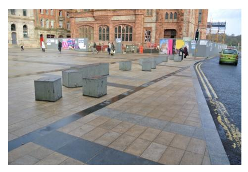
Bollards at the controlled crossing are poorly contrast and reduce the benefits of a well-designed crossing.
