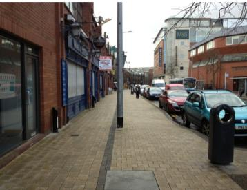
There are bollards at the northern end of Foyle Street (close to the Guildhall). The design of the bollards fails to provide an acceptable contrasting band for people with a visual impairment.
