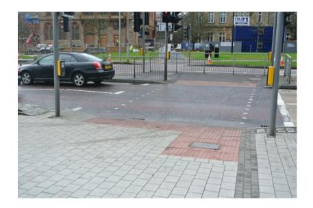
There is a broad shared use cycle/pedestrian path on Foyle Embankment with appropriate use of tactile sufaces.
