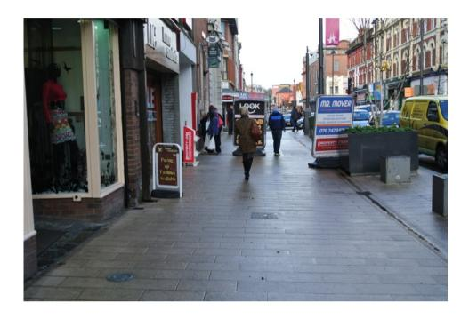
There is an in-line uncontrolled crossing at Victoria Market. Nonstandard tactile paving is used. Poorly designed bollards restrict access.
