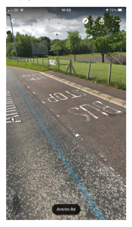
Picture shows a bus stop on the Antrim Road, Ballymena, served by Goldline coaches operating between Ballymena, Coleraine and Belfast. The footway is extremely narrow (less than 2m) with insufficient width to deploy a passenger lift. The lack of footway width would also make safe ramp access difficult.
