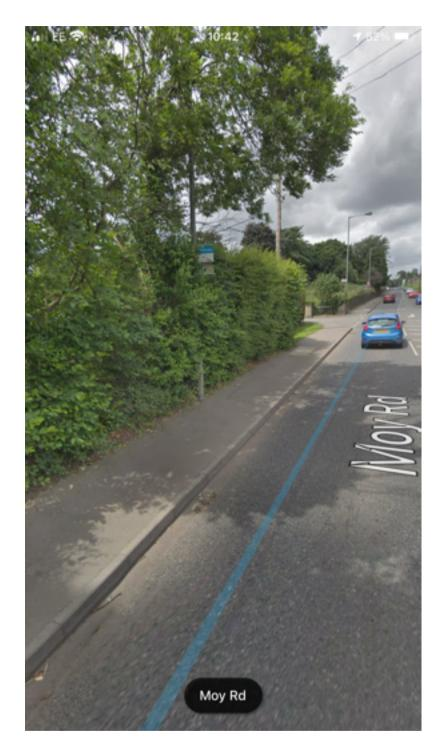
The picture shows a bus stop served by Goldline coaches on the Moy Road, Dungannon. Footway width is minimal, reduced by encroaching hedging. There is insufficient width to deploy a passenger lift but a ramp could be deployed.
