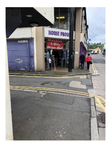
No tactile paving has been provided across The Mall at its junction with Mill Street with cobbles on the carriageway creating an unsuitable surface for many disabled people.
