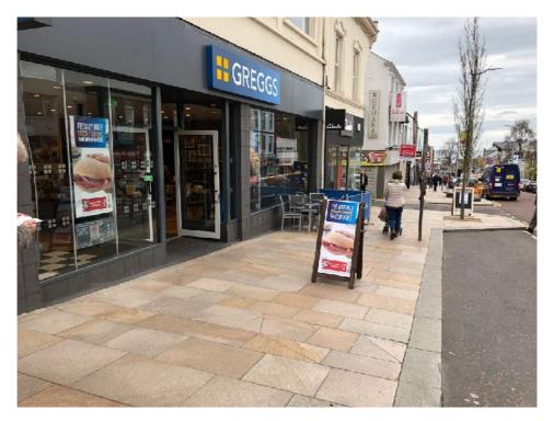
A pavement cafe further along Main Street has a good example of screening. However the cafe is located on the tactile tail of a controlled crossing and an A-Board obstructs the footway.
