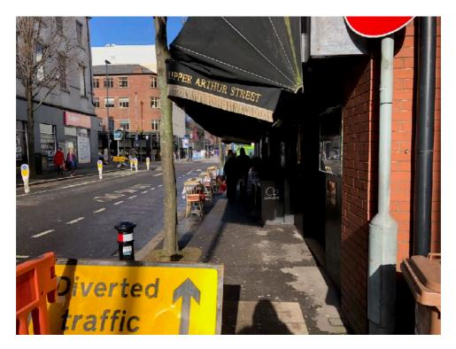
Unscreened tables and chairs associated with a pavement cafe on Chichester Street obstruct a controlled crossing. An A-Board associated with the cafe creates an additional hazard.
