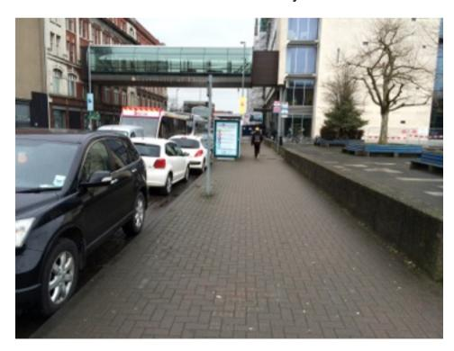
However the pavement narrows considerably at the University of Ulster Building. The steps into the building present a potential hazard to pedestrians due to poor contrasting and an absence of tactile hazard paving. The position of cycle parking also creates potential hazards.
