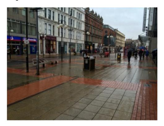
There is a good example of a controlled crossing across Royal Avenue close to the junction with North Street, although the tactile tail should extend to the building line.
