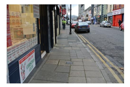
35 Kerbs have been dropped around the junction of Mill Street and Hill Street. Once again tactile paving is not provided.
