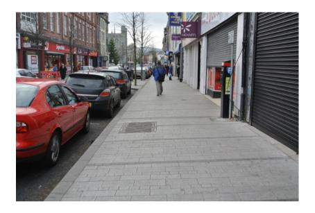
24 There is an in-line raised uncontrolled crossing on this section of Hill Street. Once again there is an opportunity to enhance pedestrian accessibility at this crossing by extending the length of the tactile paving. Bins and maintenance work are potential obstructions at this crossing.
