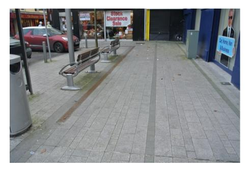
23 Proceeding up Hill Street towards Marcus Square the pavement on both sides provides a broad high quality walking surface. The kerb has been reintroduced at this point. There is a lack of consistency in the location of street furniture with parking meters located at the building line and kerb line in different locations.
