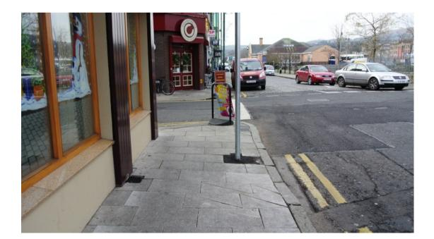
7 On the pavement at the western side of the Margaret Square there is no dropped kerb in line with the dropped kerb provided on the eastern side.
