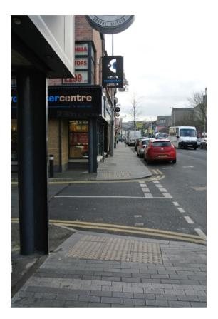
58 There is another reasonable example of an in-line uncontrolled crossing at the junction with Kilmorey Street. The utility covers do have the potential to minimise the impact of tactile on the western end of the junction.
