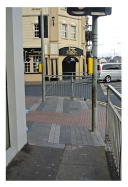
63 There are further controlled crossings across Merchant Quay and across Margaret Street. The provision at these crossings is very poor with inappropriate use of tactile paving, poor locations for control boxes and no rotating tactile cones. There are public realm improvements in the vicinity so it would be hoped that problems with the pedestrian facilities will be addressed.
